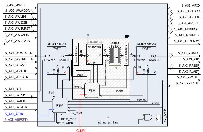
The input and output of the 2D DCT IP require more than 32 bits when N = 8, 16. This requires an Input interface to the iFIFO and an Output interface to the oFIFO. The figure shows the different interfaces for each N (4, 8, 16) when B=NO=8. As the FSM @ CLK FX controls data flow from the input and the output, it depends on N.
